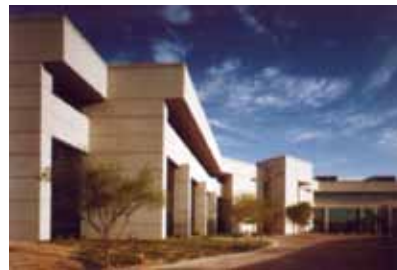
Figure 9 Cantilevered floor used to shade windows.
